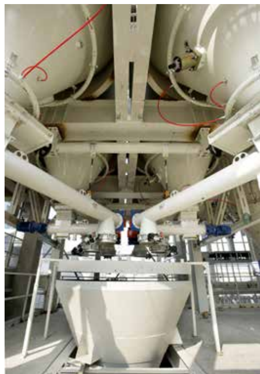
CT screw conveyors installed in industrial plant for pre-mixed powders production
